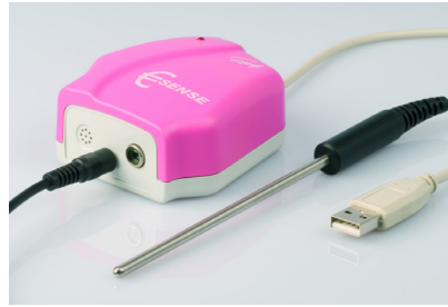
Figure 1: €Sense with plugged-in external temperature sensor and USB-connector. Also on the frontpanel: the sound sensor and the light sensor. (photography: © Andrea Denotti, denotti.com)
